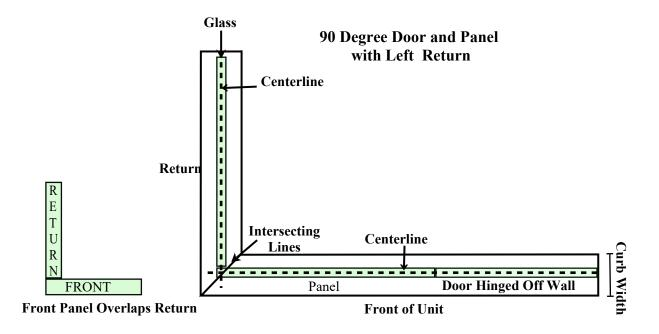
ALL measurements are to be taken from the top of the curb or from the tub deck. Not from the primary floor Unless there is a zero entry.
